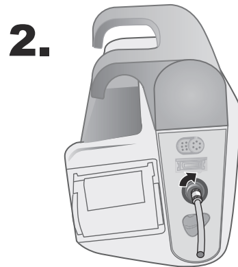
Figure 8-2 Attaching Single Lumen Hose to the X Series Unit
