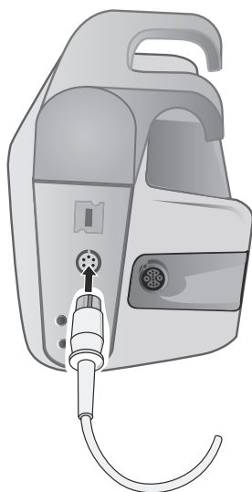
Figure 11-1 Plugging the Transducer into the X Series
