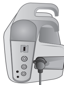
2. Connector is locked into place.
