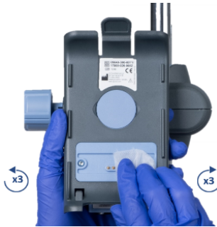
Figure 3.1. Cleaning Electrical Connectors
