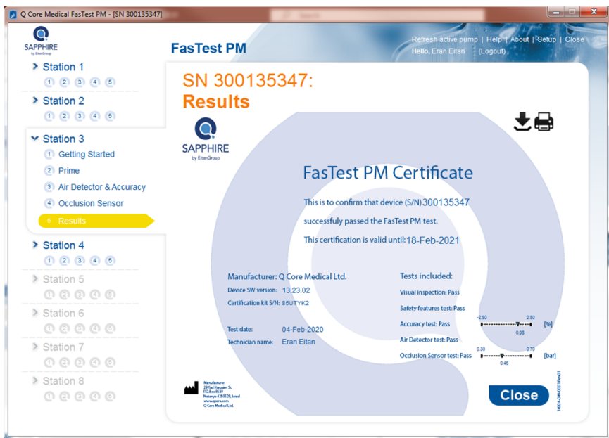
Figure 4.14. FasTest PM Results – Passed
