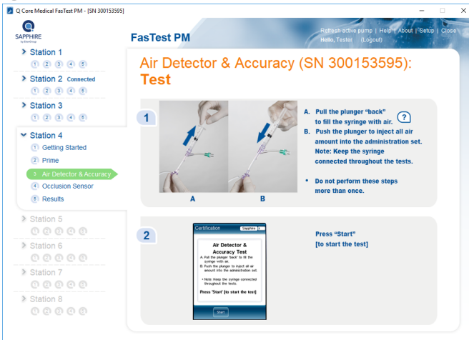
Figure 4.12. Air Detector Test
