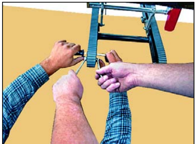
Figure 36 - Tensioning the Belt
