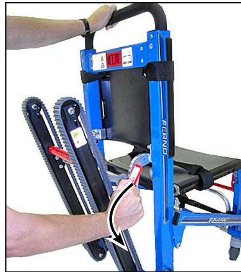
Figure 13 - Closing the Track
