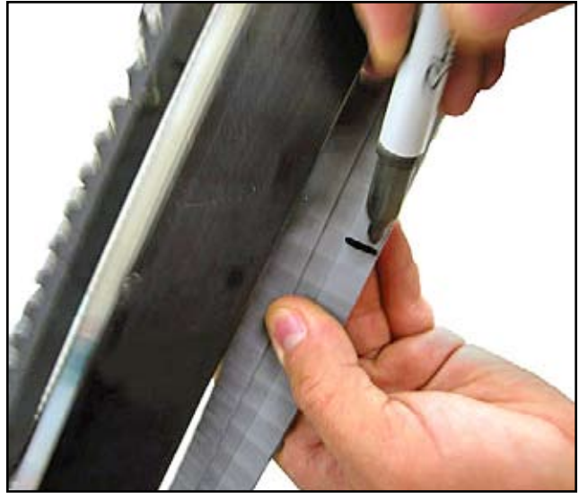
Figure 39 - Marking the Starting Point for Sanding the Belt
