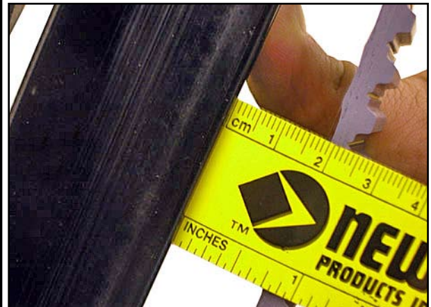
Figure 38 - Checking Tension with Chair Standing on Its Wheels
