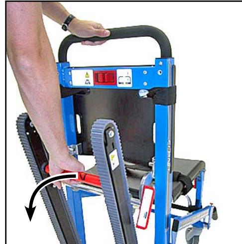
Figure 12 - Opening the Track
