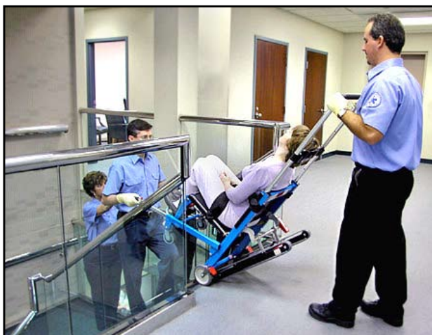
Figure 24 - Track Belts Engaging Top Step
