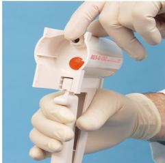
1. Test the vacuum handle before using to ensure that the unit produces a vacuum. Place a finger over the vacuum port and squeeze the handle. As the handle is squeezed, a vacuum should be felt and the handle becomes difficult to squeeze. Do not use the device if a vacuum is not felt.
